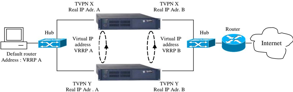
**Fig 4 : General view of a network implementing VRRP**
