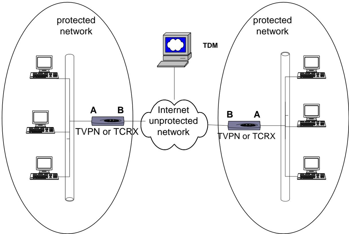
**Fig 3 : General view of a network protected by TrustWay VPN boxes**
