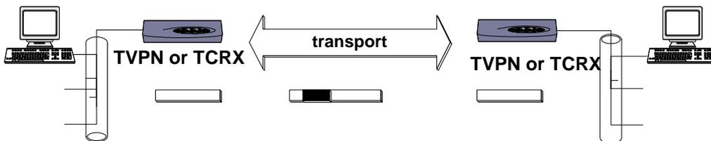
**Drop mode**: when a packet arrives if no rule (about the source and destination ) matches it (or if the drop rule is active ) then the packet is dropped.
