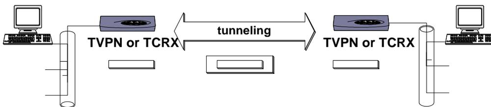
**transport mode** : all the packets for the IPSEC exchange between VPN equipments are authenticated and encrypted (but not encapsulated).
