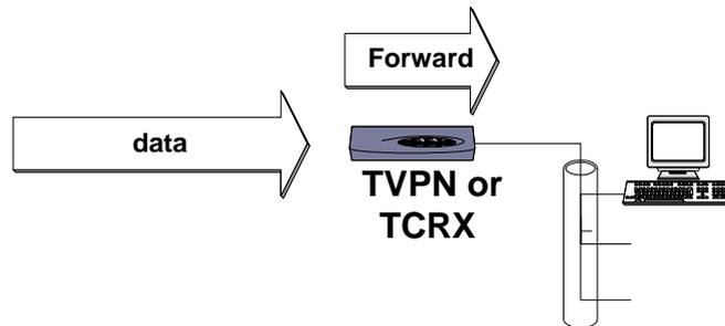
**Tunnel mode** : all the packets are encapsulated for the IPSEC exchange between VPN equipments. So the packets are authenticated and encrypted
