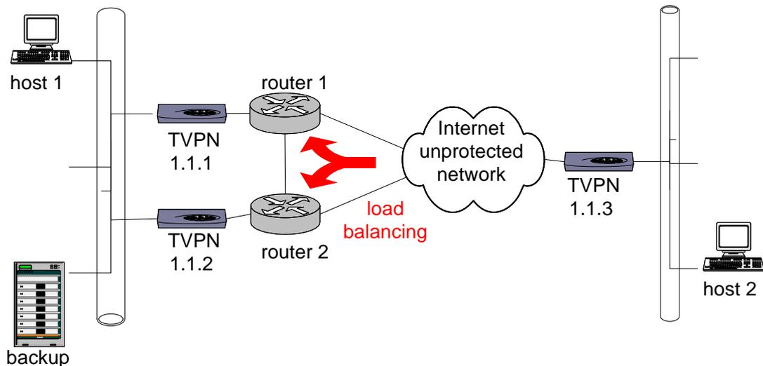
**Fig 5 : General view of a network implementing load-balancing and backup**
