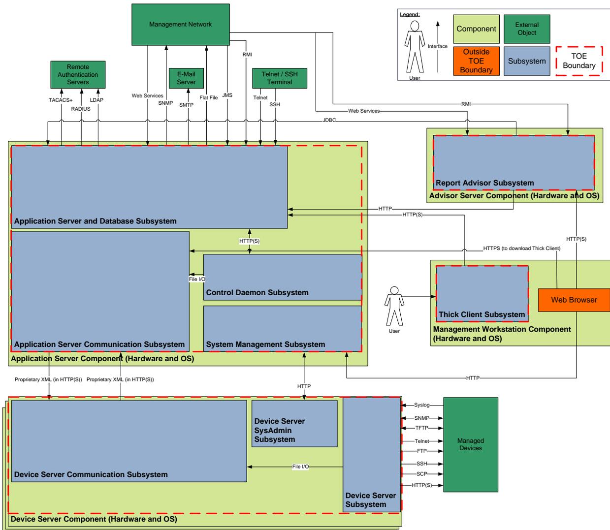
**Figure 2 - TOE and TOE Environment**
