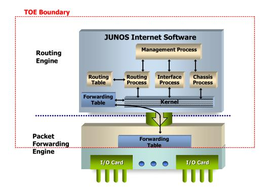
The interfaces to the TOE are twofold: the switching/routing interfaces and the management interfaces. The management interfaces include the TOE console interface through which the appliance can be managed locally and the in-band management interface via the network interfaces.
