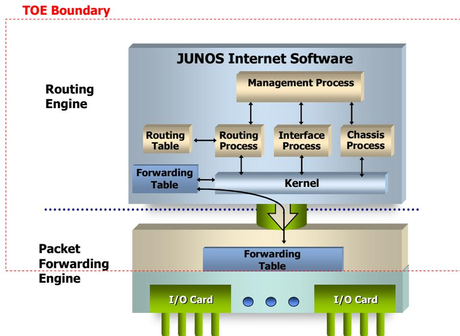
The interfaces to the TOE are twofold: the routing interfaces and the management interfaces. The management interfaces include the TOE console interface through which the router can be managed locally and the in-band management interface via the network interfaces. The M-Series routers have separate management ports, but these are outside the scope of the TOE.
