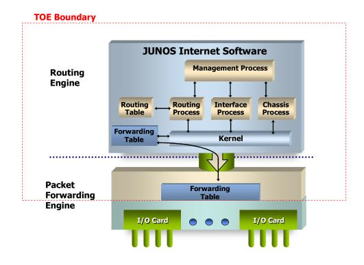
The interfaces to the TOE are twofold: the routing interfaces and the management interfaces. The management interfaces include the TOE console interface through which the appliance can be managed locally and the in-band management interface via the network interfaces. The M-Series and T-Series routers have separate management ports, but these are outside the scope of the TOE.
