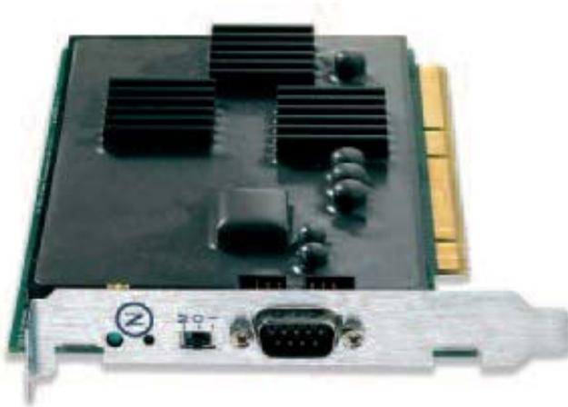
In addition to the PCI connection to a server, the HSM also supports a connection to a smart card reader. Smart cards may be used to hold logical tokens used to encrypt key blobs. Possession of the correct smart card provides authorization to use the stored key.
