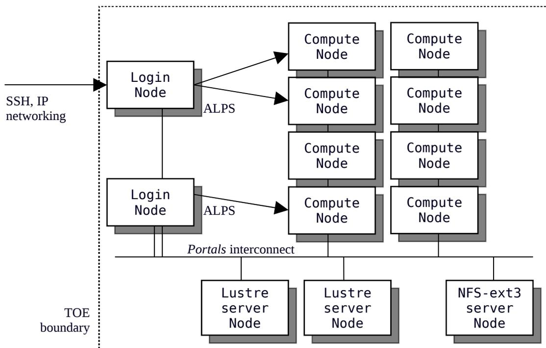
Users can login to *login nodes* using the *ssh* protocol, and use the Application Level Placement Scheduler (ALPS) to submit noninteractive jobs for execution on *compute nodes*. The compute nodes do not permit direct login.
