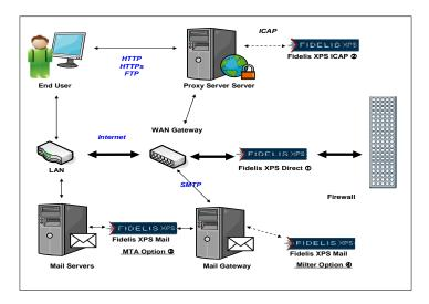
The physical boundary of the TOE is the Fidelis XPS appliance. As indicated above a given Fidelis XPS configuration includes a CommandPost appliance and one or more Fidelis XPS sensor appliance. Each of these components is a self-contained hardware device.
