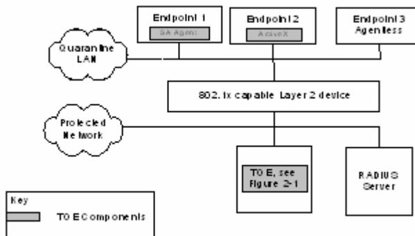
**Figure 2-4 Evaluated Configuration for 802.1X Enforcement Method**
