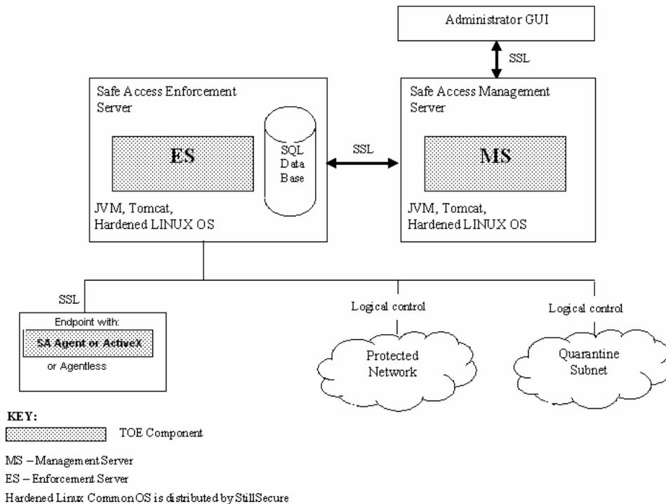
**Figure 2-1 Safe Access Server Components and Logical Relationship to the Network Components**
