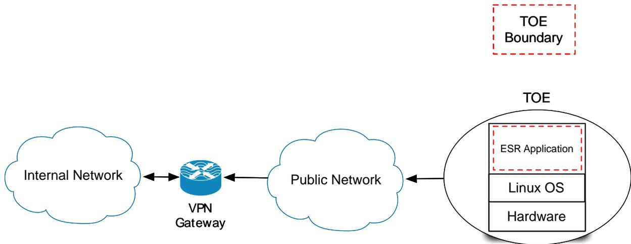
The following figure provides a visual depiction of an example TOE deployment. The TOE boundary is surrounded with a hashed red line.
