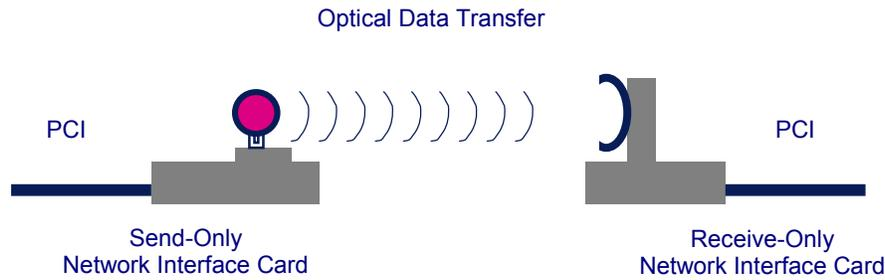
**Figure 1 - High Level view of the Data Diode Interface**
