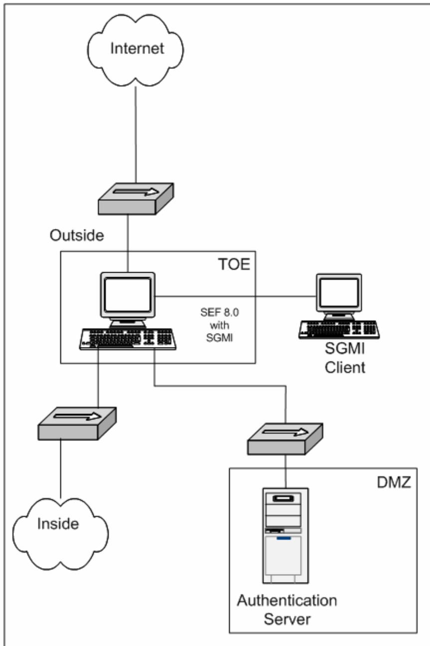
**Diagram 2-1: The Symantec Enterprise Firewall Network Configuration**
