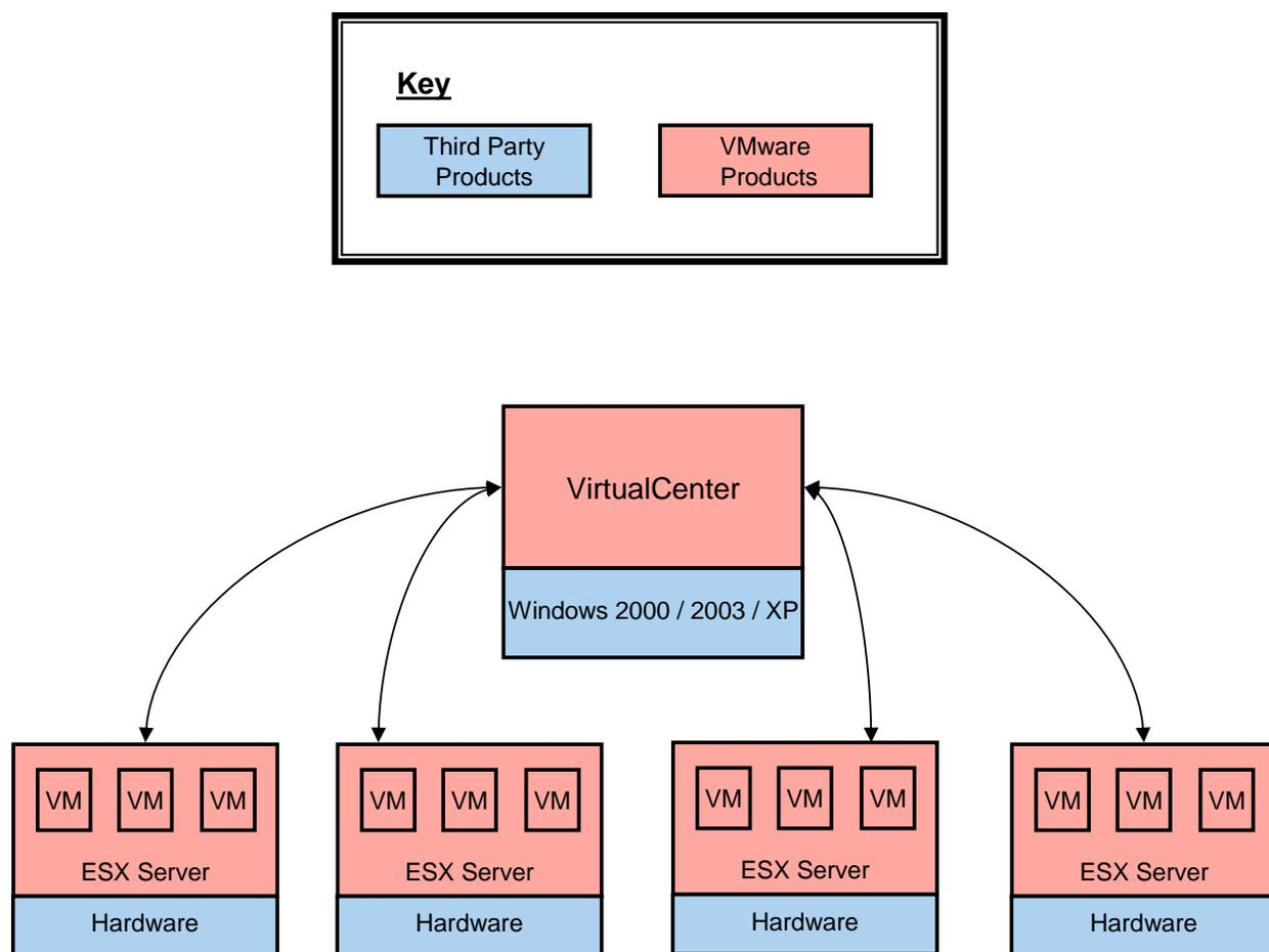
Figure 1 - Deployment Configuration of the TOE
