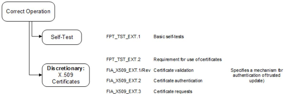
Figure 16: Correct Operation SFR Architecture
