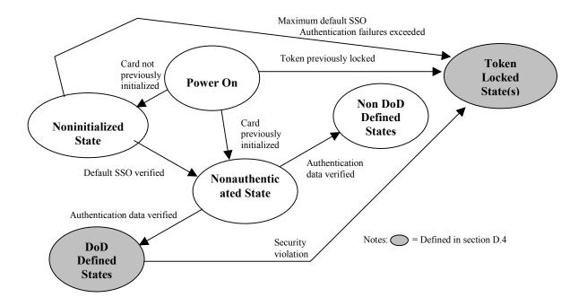
Figure D-1 Token Top Level State Diagram
