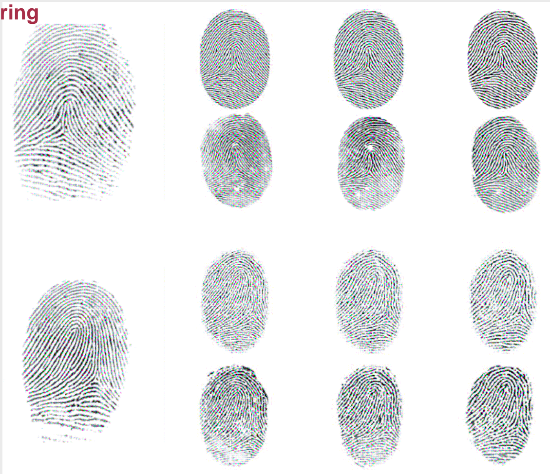
Original fingerprints (left). Reconstructed images without noise (row 1) and with noise (row 3). The respective final fake fingerprints without noise (row 2), and with noise (row 4)
