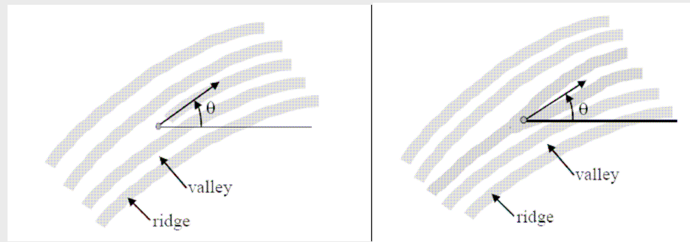
Minutia placement on a ridge ending (left) and on a ridge bifurcation (right).
