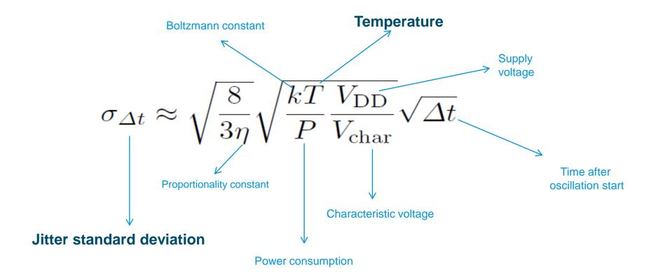
Above is for a single-ended CMOS RO derived by Hajimiri et al. – "Jitter and Phase Noise in Ring Oscillators", IEEE J. Solid-State Circuits 34(6) (1999) 790-804. (Reference for equation and figure on prev slide)
