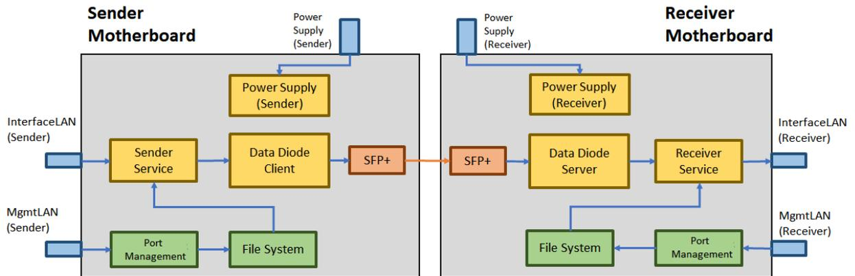
\*Power Supply (Sender) module supplies power to all modules in the Sender Motherboard. Similarly, Power Supply (Receiver) module supplies power to all modules in the Receiver Motherboard. The connections between the Power supply modules and their corresponding modules are omitted in the diagram to keep the diagram readable.
