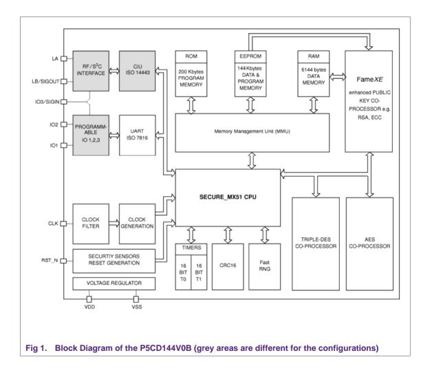
There are differences in the configurations, indicated in grey in the figure. Refer to section 2.2 for information about the configurations. The following tables list the TOE components.
