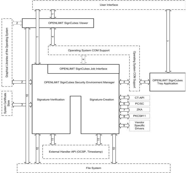
Figure 1: Decomposition of the main components of the TOE
