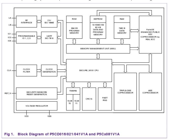
The TOE consists of the IC hardware and the IC Dedicated Software as composed of IC Dedicated Test Software and IC Dedicated Support Software. All other software is called Security IC Embedded Software and is not part of the TOE.
