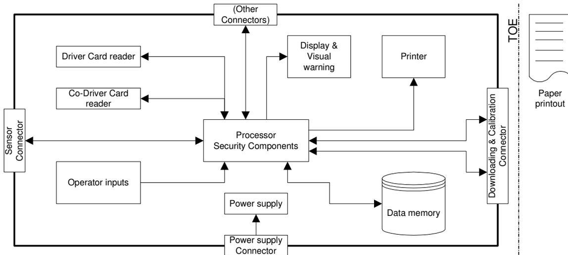
Figure 1 Digital Tachograph DTCO 1381
