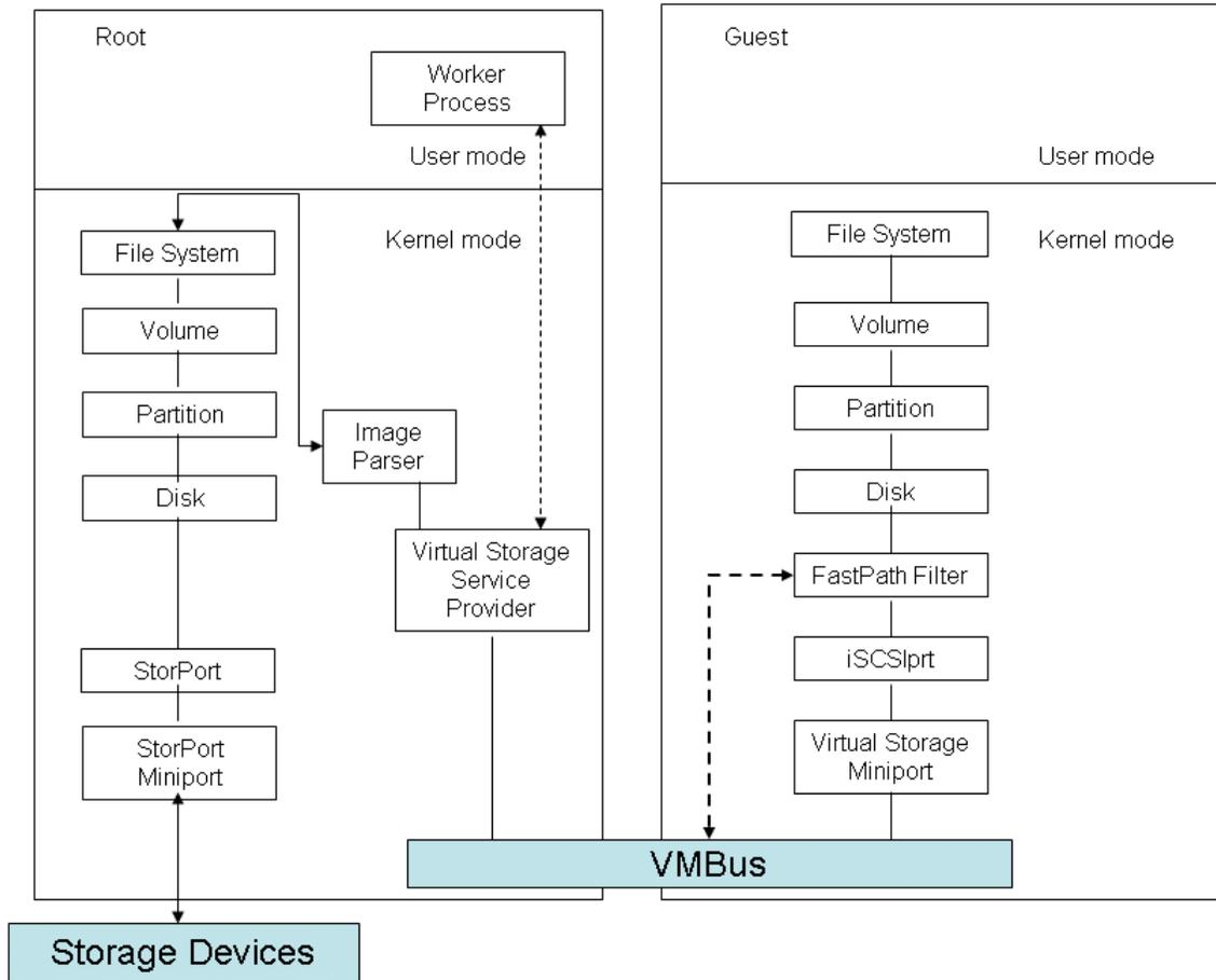
Figure 2: Example of a flow for access to a virtual hard disk (VHD)
