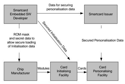
Figure 5: ROM Mask and initialisation data delivery
