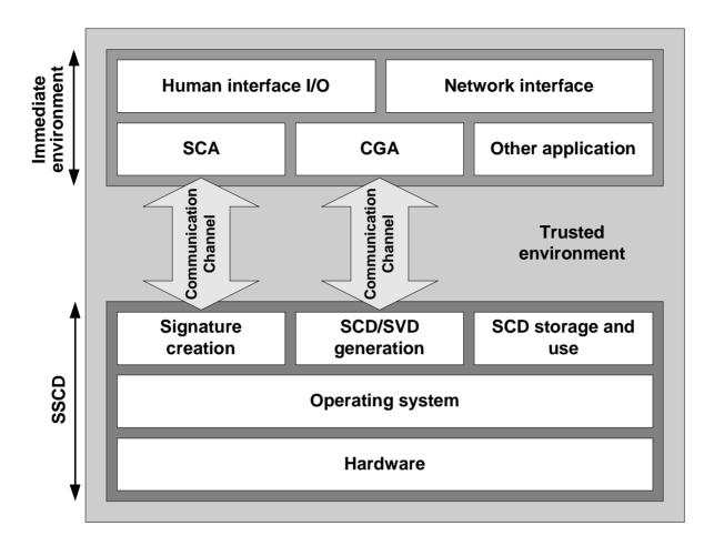
Figure 1: Scope of the SSCD, structural view
