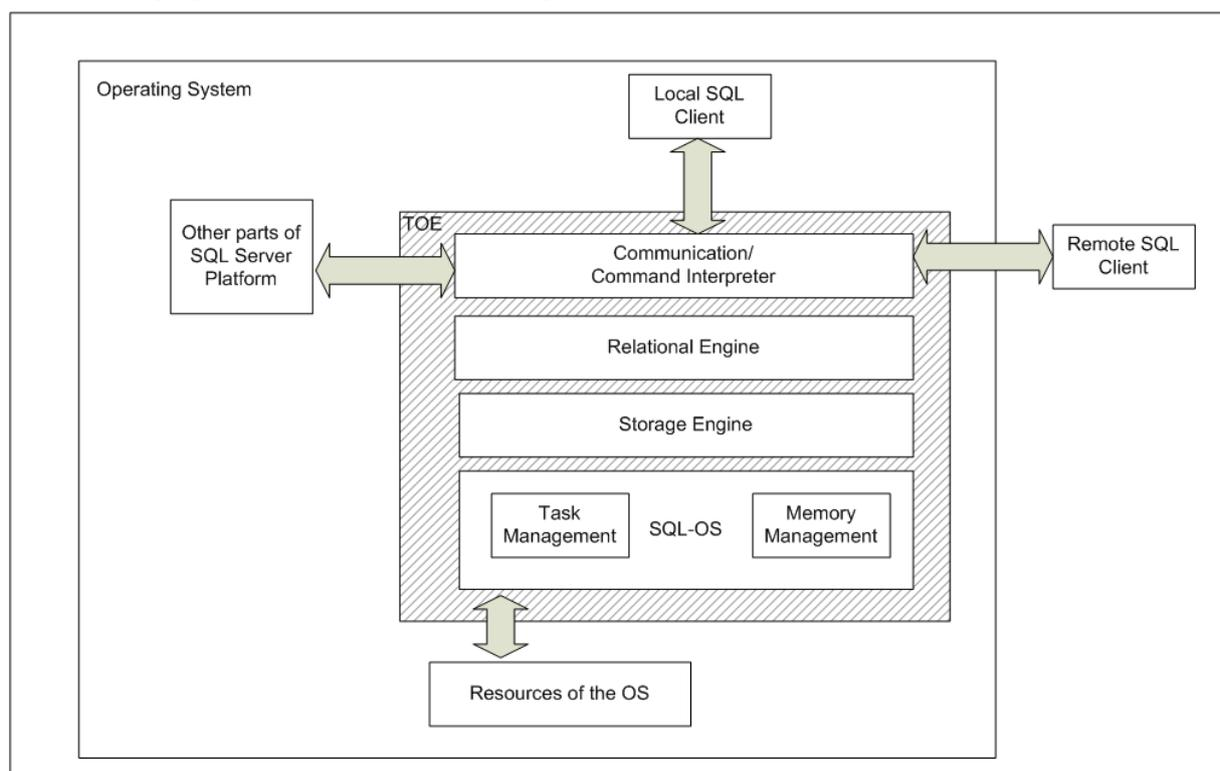
**Figure 1 - TOE structure**
