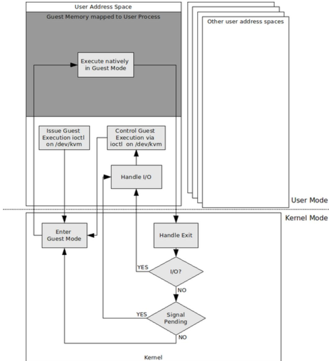
When the kernel releases control of the CPU to the virtual machine process, it sets the processor state of the CPU to the user state when calling the regular application logic in user mode. However, when returning control of the CPU to the guest code, the CPU can be set either to supervisor state or user state, depending on the state of the CPU when the Linux kernel initially obtained control.
