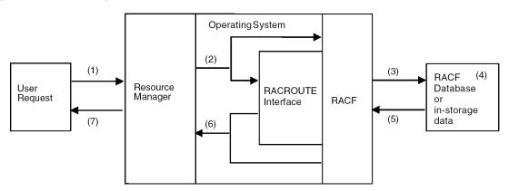
A program that wants to access a resource uses a function that is part of the external interface provided by the z/OS operating system to one of the z/OS components (1). An example is a program that wants to open a data set.
