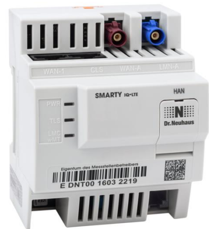
Figure 3: SMARTY IQ-LTE casing and external interfaces
