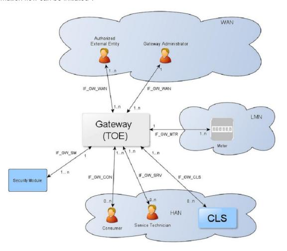
Figure 2: The logical interfaces of the TOE
