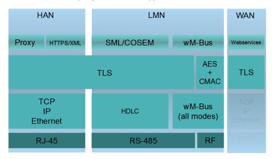
Figure 4: The TOE's protocol stack
