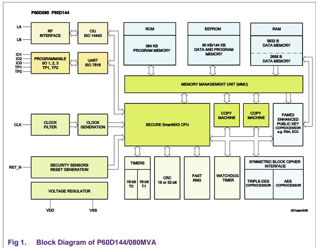
Fig 1. Block Diagram of P60D144/080MVA
