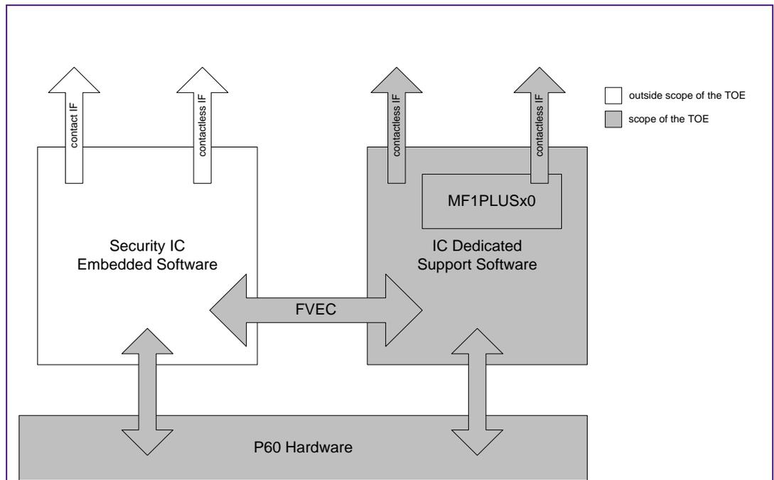
Fig 2. Logical boundary of the TOE
