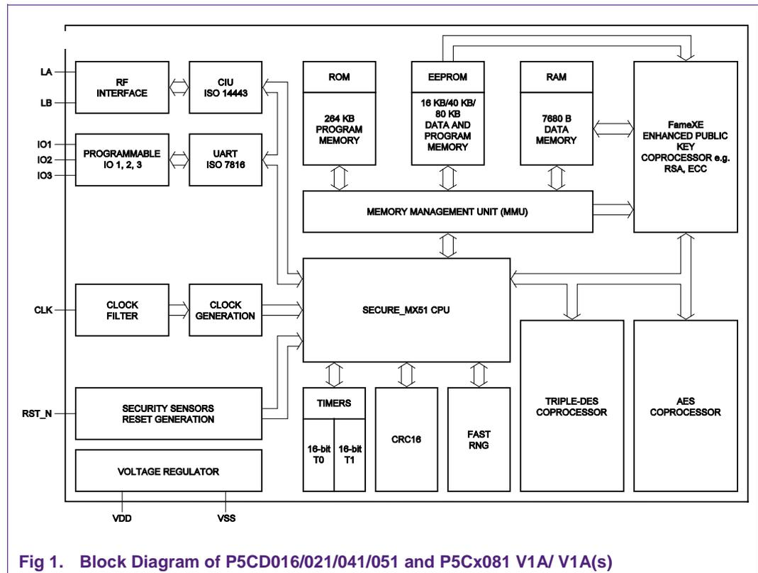
Fig 1. Block Diagram of P5CD016/021/041/051 and P5Cx081 V1A/ V1A(s)
