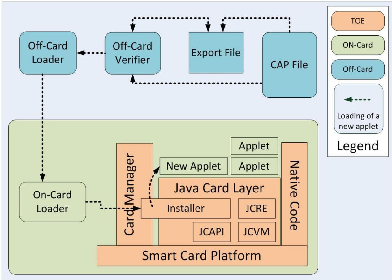
Figure 3 Java Card Platform and applet installation environment
