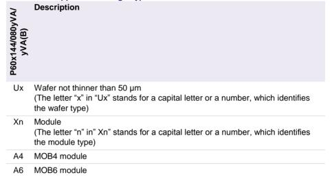
For example, commercial type name P60D144MX0/9Arrff2 denotes major configuration P60D144MVA with MIFARE Plus MF1PLUSx0 supporting 2 kBytes of EEPROM and PDM1.1 dual interface smart card module. The characters 'rr' and 'ff' are individual for each customer product.
