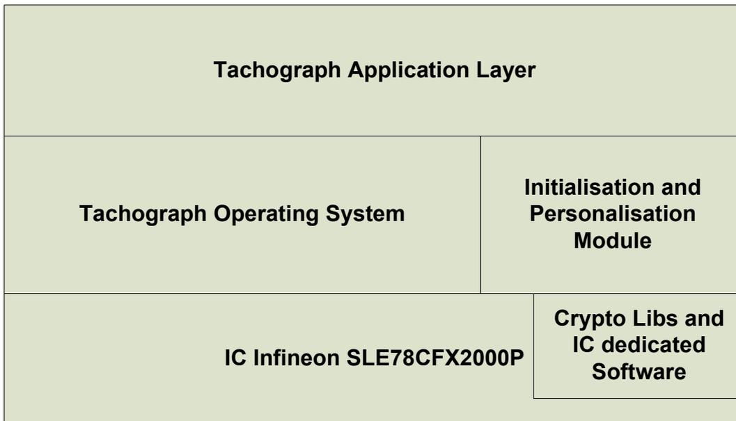
**Figure 1: TOE Architecture**
