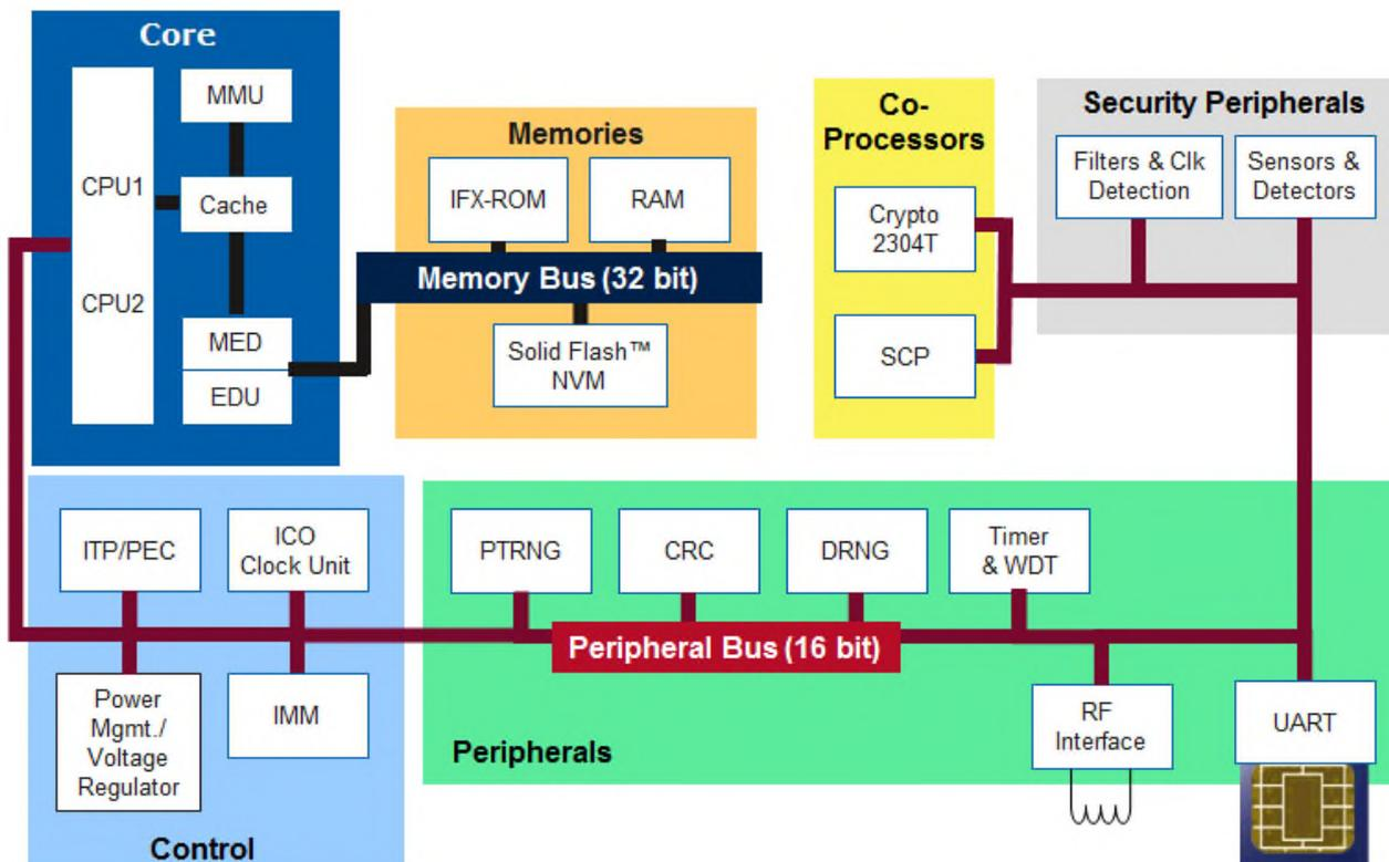
The major components of the core system are the dual CPU (Central Processing Units) including the internal encryption leaving no plain data anywhere, the MMU (Memory Management Unit), the MED (Memory Encryption/Decryption Unit) and the CACHE memory.
