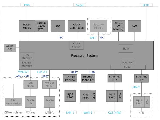
Figure 1.6: The hardware parts of the TOE
