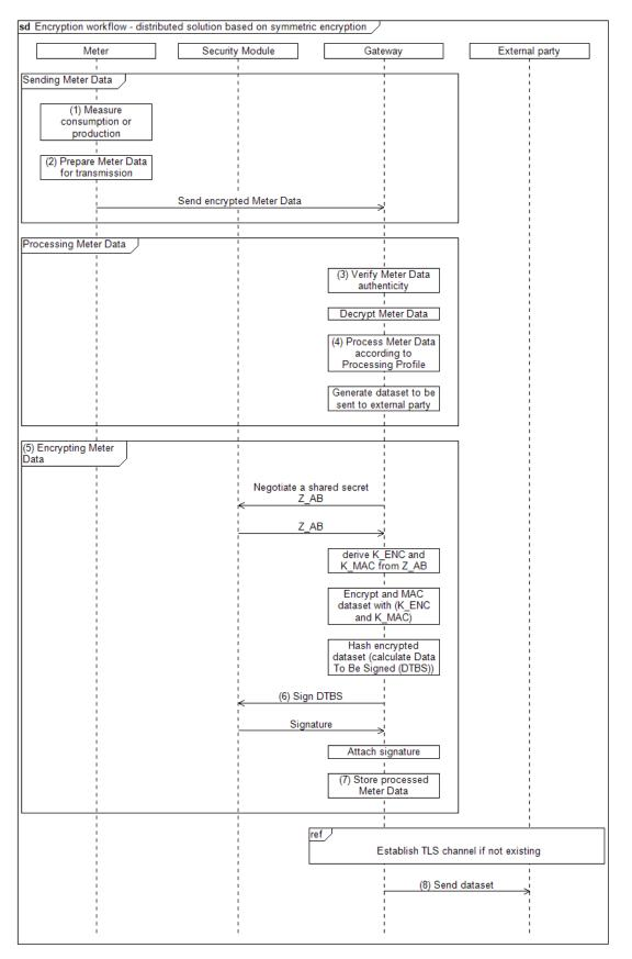
Figure 1.7: Cryptographic information flow for distributed Meter and Gateway
