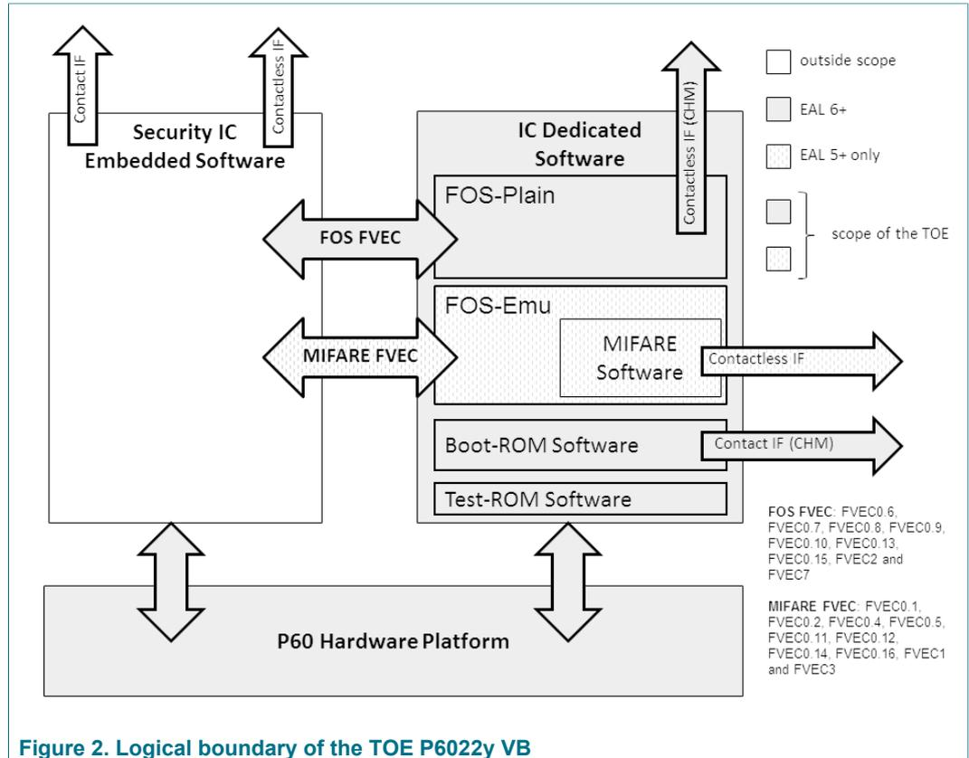
Figure 2. Logical boundary of the TOE P6022y VB
