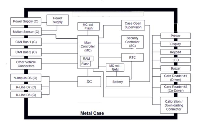
Figure 4: EFAS-4.5 V03.00 with Interfaces
