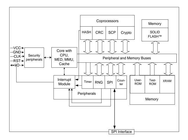
Figure 1: Block diagram of the SLB9670\_2.0
