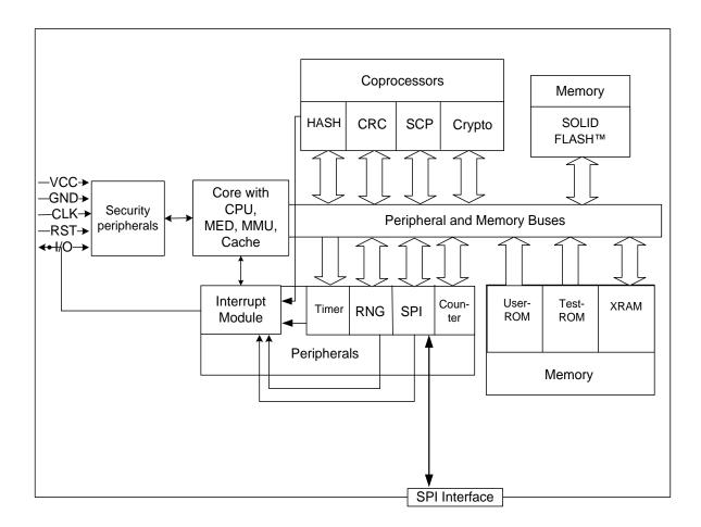
Figure 1: Block diagram of the SLB9670\_2.0
