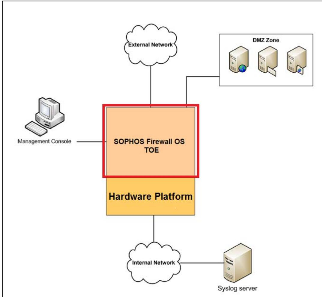
Figure 2: TOE Physical scope and boundary
