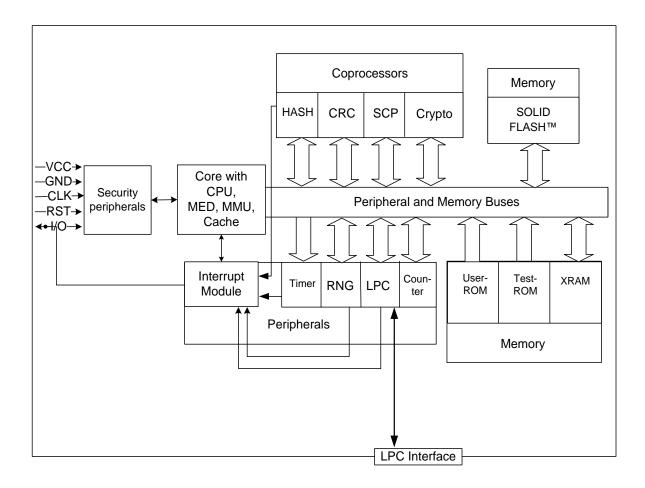
Figure 1: Block diagram of the SLB9665\_2.0
