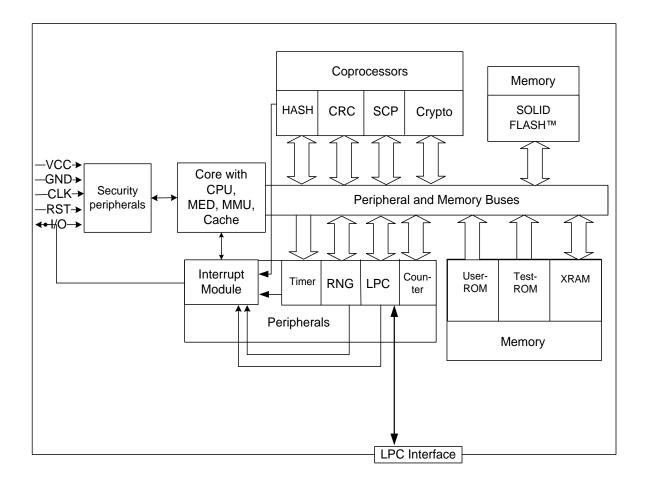
Figure 1: Block diagram of the SLB9665\_2.0
