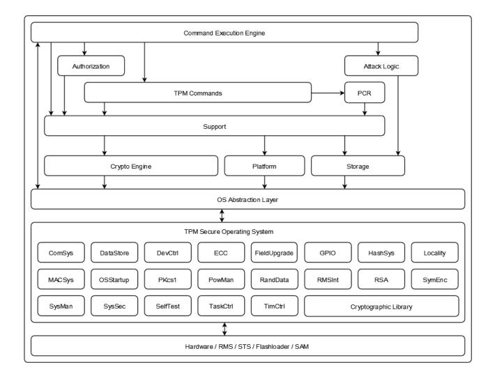
Figure 2: Firmware block diagram of the SLB9665\_2.0
