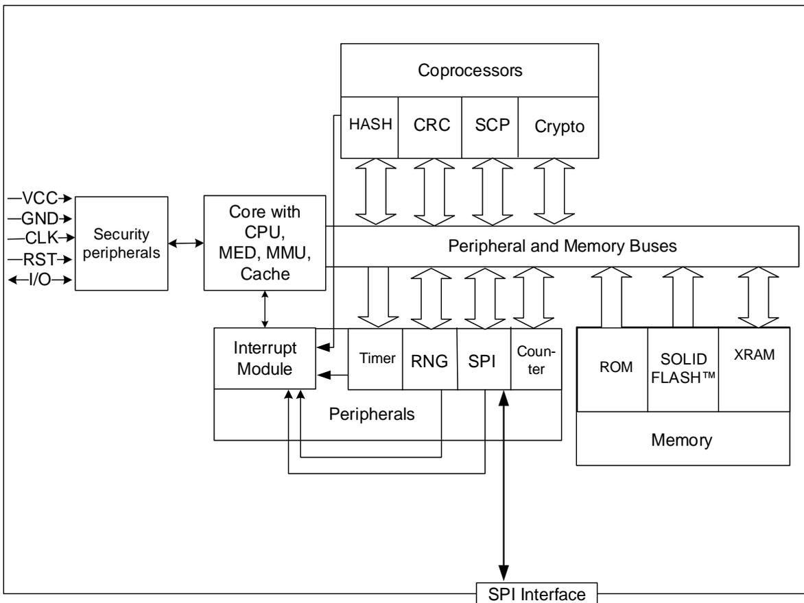
Figure 1: Block diagram of the SLB9670\_2.0
