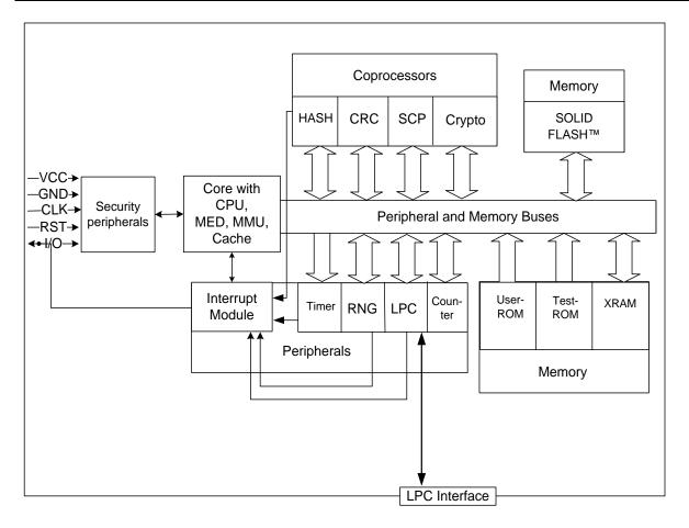
Figure 1: Block diagram of the SLB9665\_2.0
