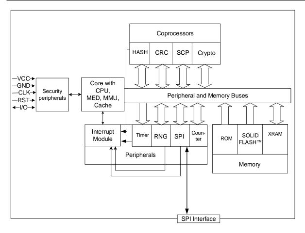
Figure 1: Block diagram of the SLB9670\_2.0
