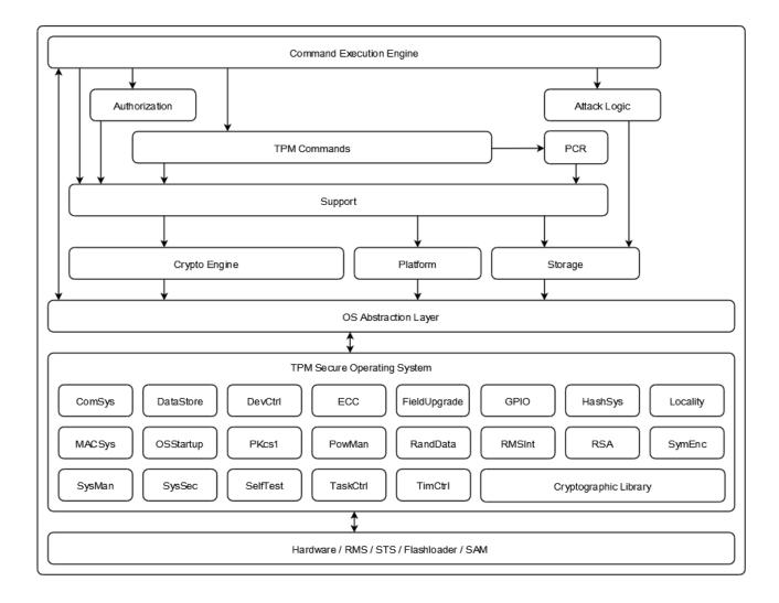
Figure 2: Firmware block diagram of the SLB9670\_2.0
