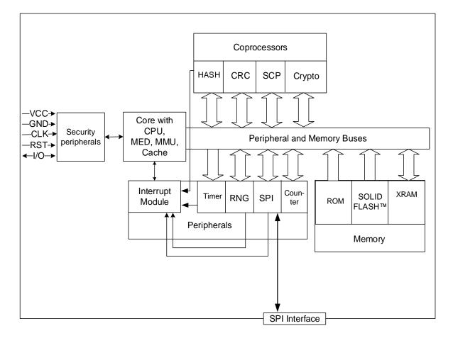
Figure 1: Block diagram of the SLB9670\_2.0
