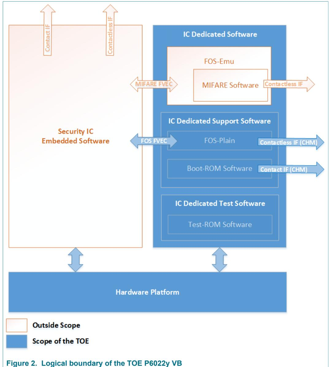
Figure 2. Logical boundary of the TOE P6022y VB
