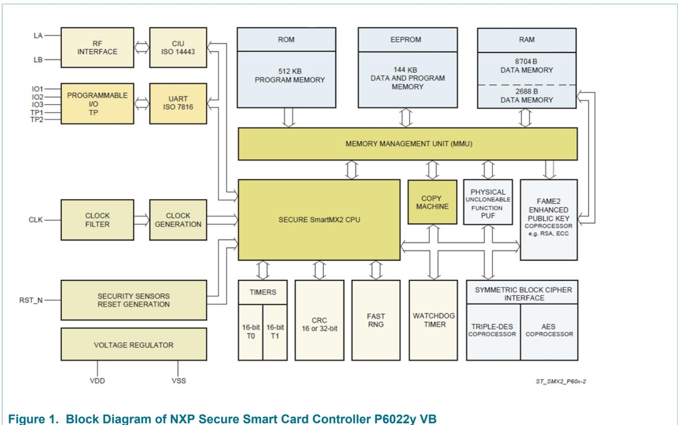
Figure 1. Block Diagram of NXP Secure Smart Card Controller P6022y VB
