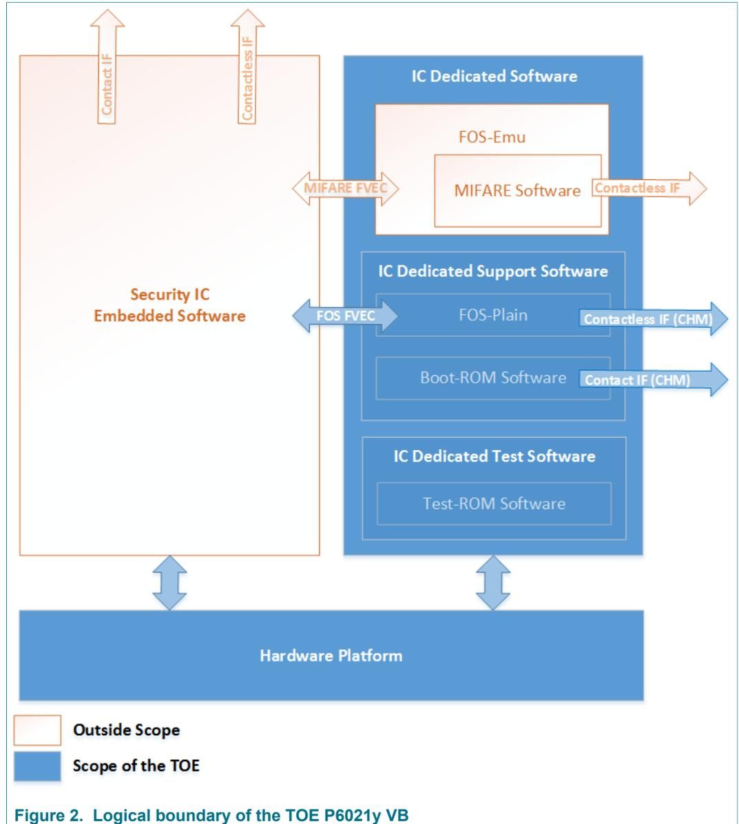
Figure 2. Logical boundary of the TOE P6021y VB
